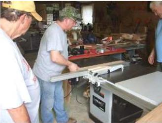
We cut the pieces to width using the table saw.
