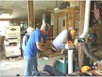
Then we started prepping the wood using the jointer and planer.
