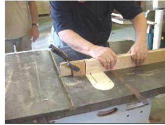
miter gauge with a stop block to establish the tenon length. Then we clamped the test piece in the tenon jig and adjusted
