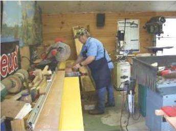
And then to length using a sliding compound miter saw.
