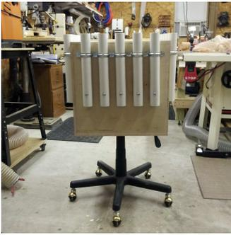
Mark Underwood designed, and Waid Gauthier made, this mobile tool rack for his lathe tools and supplies. It's mounted on an old swivel office chair pedestal. It has
