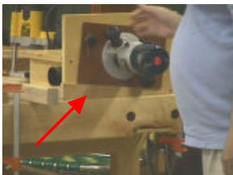
router table that works really well for cutting tenons. It has a wedge adjustment for the bit height that
