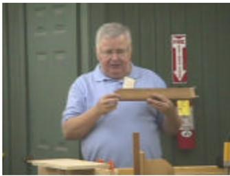
To eliminate splinters, John likes to use his table saw, with a sled, to score the wood on all four surfaces – even if
