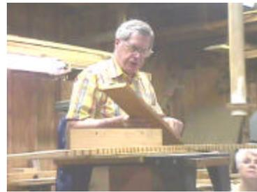
moldings along with the jig he uses to cut them. Dick normally uses his router to cut the moldings,
