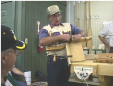
Jerry Shivers made a clamping jig to help him glue up mitered corners.
