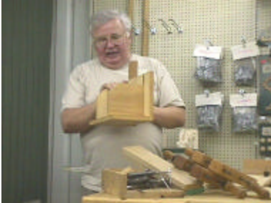
And a jig he uses to cut tenons for his table saw
