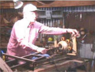
Lyman made his own boring bar from 1" square tubing. It's basically a large frame with a long bar on one side. A replaceable cutting tip (usually like a round nose scraper) is mounted on the end of the bar. A special steady
