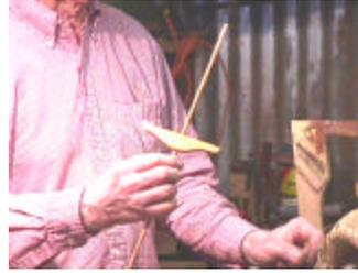
homemade gauge consisting of a crosshead with a hole, a dowel and a screw to tighten the crosshead to the dowel. Commercial versions are also available from woodworking catalogs.
