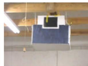
Don built a homemade air cleaner for his shop. He built a plywood box with a large hole on each side.
