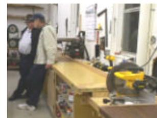
long table along one wall so he can safely cut long boards on his radial arm saw and compound miter
