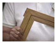
widths. His solution: Half-lap miter joints – they provide the needed 'face grain' gluing
