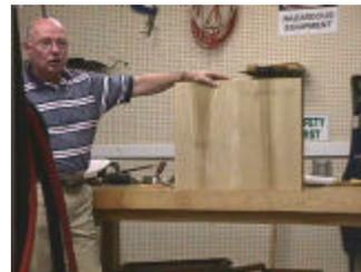
an adz. After he gets the rough shape, he does the final shaping with an inshave or travester tool and a disk sander. When the shaping is finished, he cuts the seat profile out and does final shaping of the edges.
